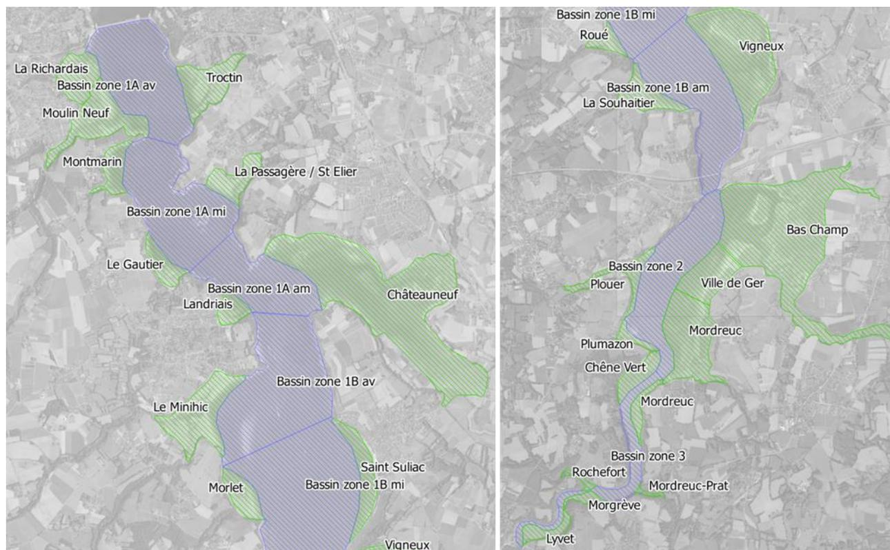
**FIGURE 17 – PROPOSITION DE DECOUPAGE DU BASSIN EN ZONE DE DRAGAGE**
