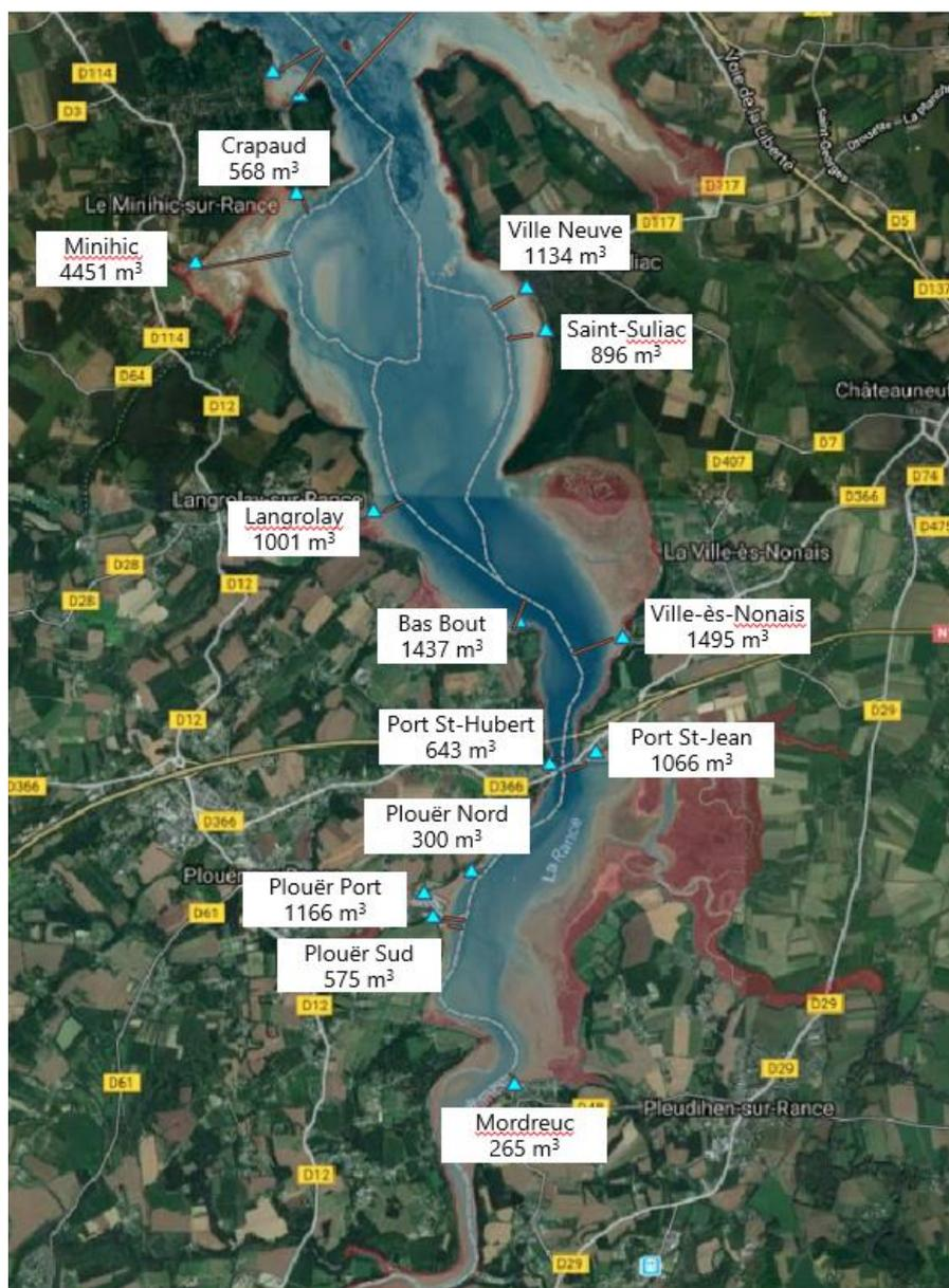
FIGURE 30 – VOLUMES DE DEPOTS RECENTS (2011-2018) CALCULES SUR LES ZONES D'ACCES DU CHENAL AUX CALES DE MISE A L'EAU
