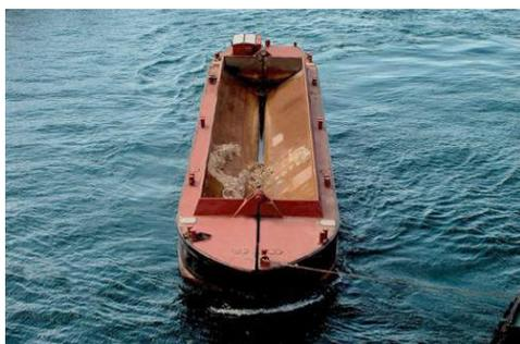
FIGURE 47 – IMMERSION DE SEDIMENT A L'AIDE D'UN CHALAND FENDABLE
